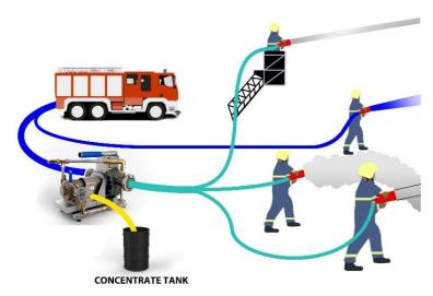
FIREMIKS enables central mixing of extinguishing agents to several nozzles placed at different lengths and heights from FIREMIKS, handled independently from each other. Dosing is immediate which allows quickly opening and closing the nozzles (pulsing).
