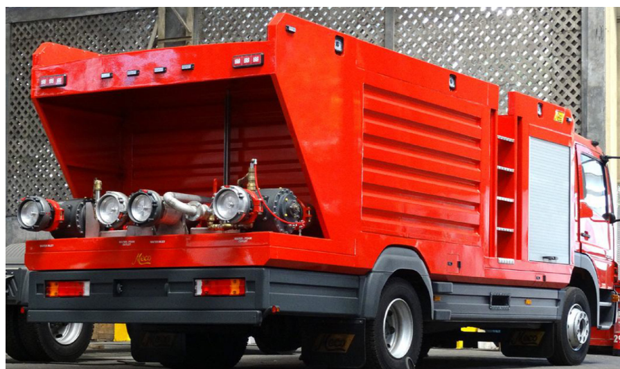
▼ Two FIREMIKS FM 8000-3-GP-F installed at two Pertamina Oil Fire trucks in Indonesia.
