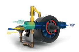
The water flow goes through the FIREMIKS water motor. This generates a circular rotor motion that is transferred to the pump through the direct-drive coupling. The concentrate is pumped into the water motor outlet, where dosing occurs.
