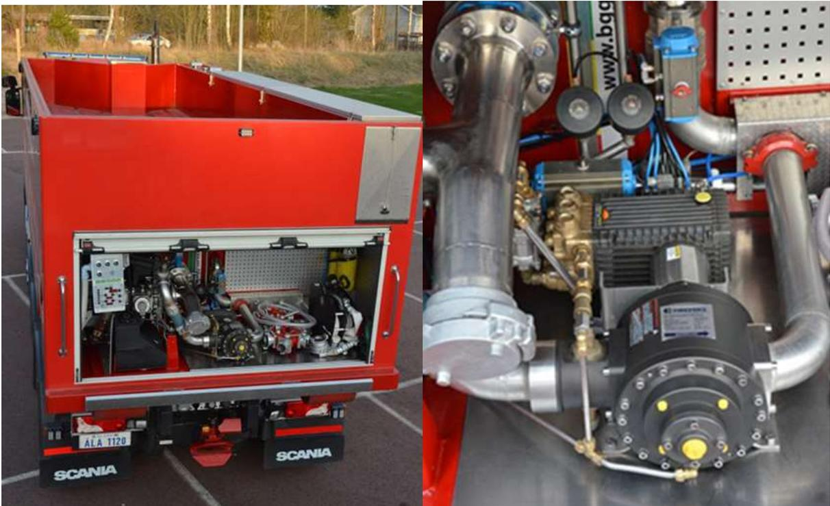
**Finland, Åland Island, Jomala Fire Brigade - FIREMIKS 1800-0,3-0,6-1-PP-F** mounted on a 24-tonne multi-lift system with two 200-litre foam concentrate tanks and a 15,000 litre water tank, with an additional 7,000 litre open pool on the roof. The unit offers three selectable dosing rates 0,3%, 0,6% and 1% and is intended to be used specifically for the local airport and large-scale fires on the island.
