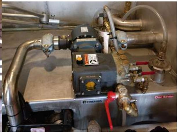
**Sweden, Medelpad Fire Brigade - FIREMIKS 400-1-2-3-PP-F** on a multi-purpose hook-lift system. Flow 100 – 400 lpm, dosing rate selectable 1%, 2% and 3% of X-fog concentrate to be used with hand-held nozzles.
