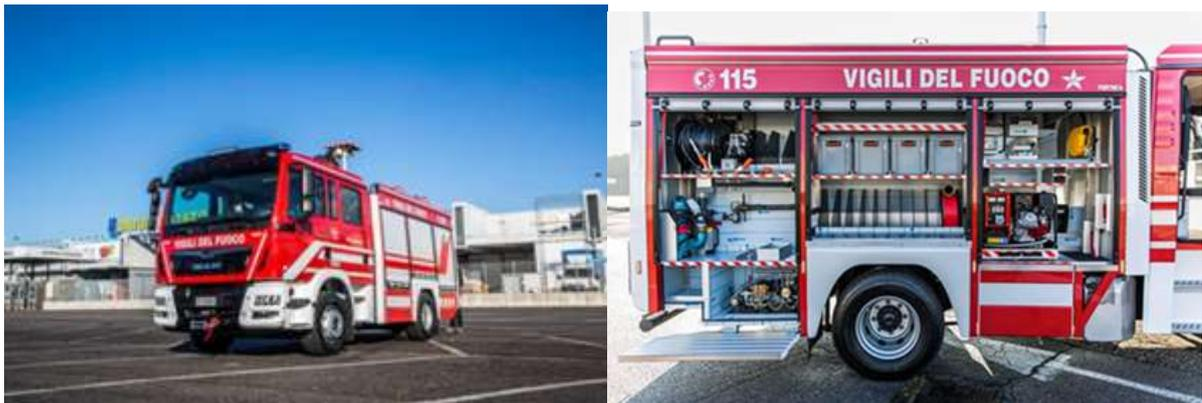
**Italy, Vigili del Fuoco, Lumezzane – Brescia - FIREMIKS 450-1-2-3-PP-M-ALU installed in a MAN truck, to be used Mobile. Flow range 100-450 lpm and selectable dosing rate 1-2-3%, max pressure 16 bar.**
