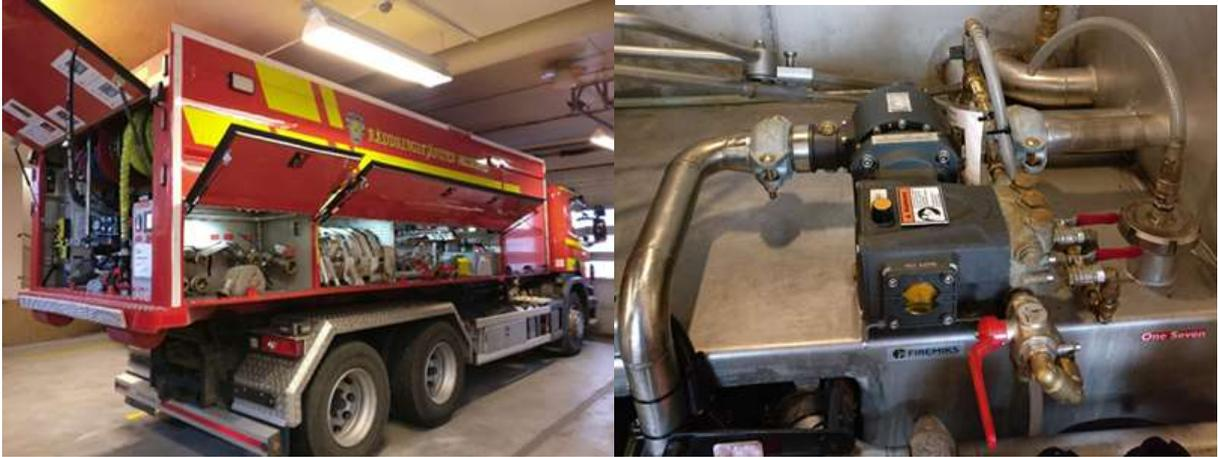
**Sweden, Medelpad Fire Brigade - FIREMIKS 400-1-2-3-PP-F** on a multi-purpose hook-lift system. Flow 100 – 400 lpm, dosing rate selectable 1%, 2% and 3% of X-fog concentrate to be used with hand-held nozzles.
