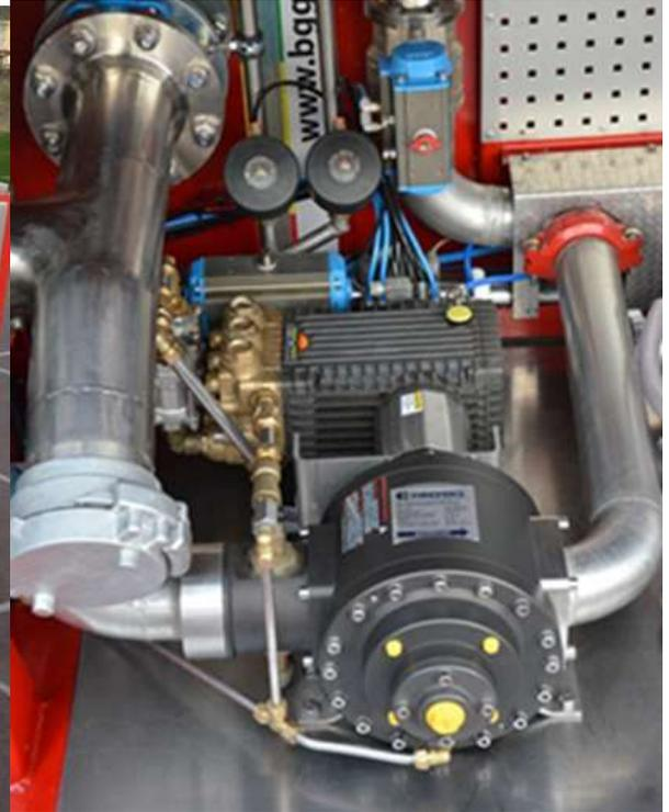
**Finland, Åland Island, Jomala Fire Brigade - FIREMIKS 1800-0,3-0,6-1-PP-F** mounted on a 24-tonne multi-lift system with two 200-litre foam concentrate tanks and a 15,000 litre water tank, with an additional 7,000 litre open pool on the roof. The unit offers three selectable dosing rates 0,3%, 0,6% and 1% and is intended to be used specifically for the local airport and large-scale fires on the island.
