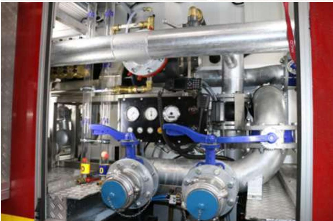
**Lithuania, Fire truck built by Iskada for PKN Orlean's refinery in Mazeikiu**, Renault C 430 6x4 double cab. 4000 liters of water, 2000 liters of foam concentrate. Water pump: JOHSTADT NP6000S 6000 l/min at 10 bars. **FIREMIKS 4800-3-PP-F-ALU** with flowrate up to 4800 l/min, 3% dosing rate.
