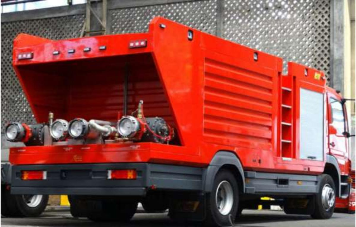
**Indonesia, two Foam trucks built by PT Meco Inoxprima for Pertamina, State oil company, each truck equipped with 2 x FIREMIKS 8000-3-GP-F-ALU, giving total 16,000 lpm capacity of dosing 3% concentrate.**
