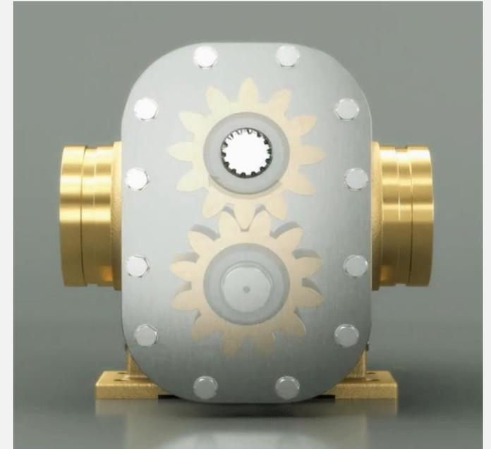
A gear pump uses internal gears to grab the concentrate. The advantages of using gear pumps are that flow is not pulsating, and the pump "grip" very well both high and very high viscosity concentrates.
