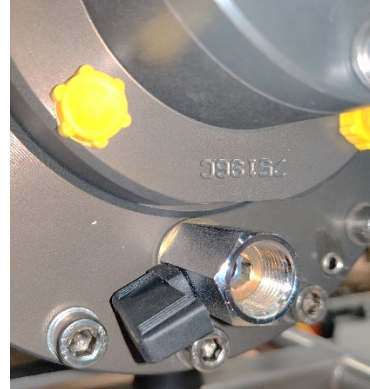
Drain valve Open
